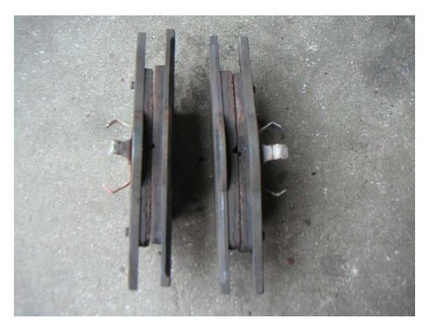
To our surprise, the pads using our bushings wore MORE than the pads without. How could this be?
