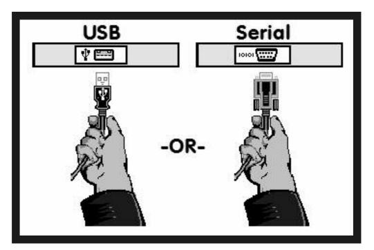
▲ Connect the Serial end of your Serial Interface or the USB end of your USB Interface to the correct port on your PC. If your PC is further from the vehicle than 6 feet, connect an approved Extension Cable between the PC and the Interface. This is included in the Pro-Kit.
