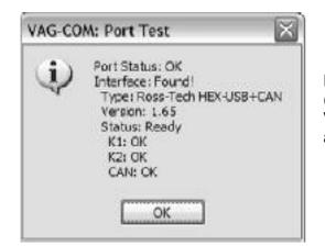
◄ Select the correct port for your PC's Serial Port (typically COM1 or COM2) or USB Port (USB) and click the **[Test]** button. Ensure that VAG-COM finds your interface. You should see a message like this.
